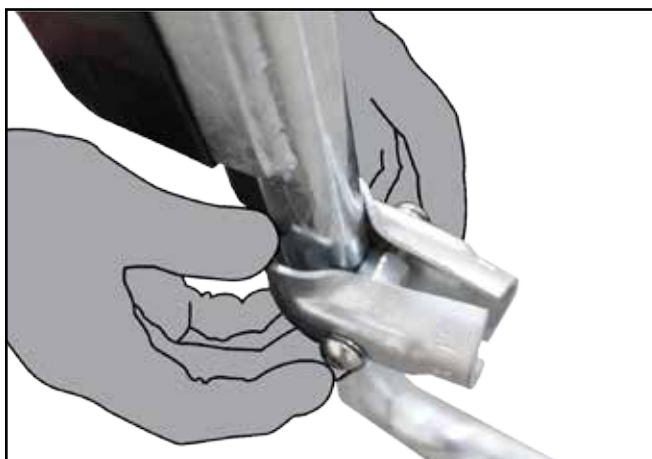
GB - O. Mount clamp on lower part of gate, just above the bend and insert mid rail. Use 6mm hex head socket to tighten supplied M10 bolts into coupling nut.
